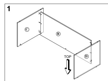
Turn Top Panel (A) upside down and insert Cam Lock pins (1) into top panel and into side panels (C,D). Insert Klix Cams (2) in Side Panels (C,D) and back panel (B). Attach Back Panel (B) to side panels (C,D) and Top Panel (A). Turn Klix Cam to tighten.
